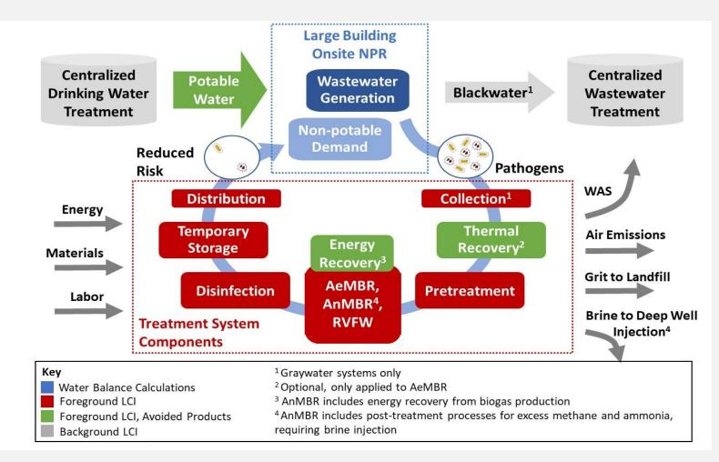
Analyze cost and environmental impact of systems treating mixed wastewater and source separated graywater for onsite NPR (0.01-0.016 MGD). Integrated results with microbial risk assessment.
